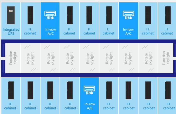
Integrated UPS cabinet: UPS inside modular data center
