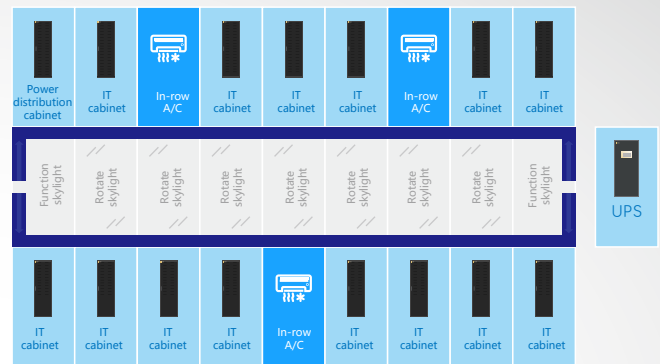
UPS outside of modular data center
